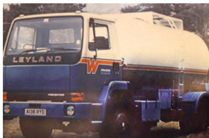
Because milk is pumped at atmospheric pressure, the tank design does not need to comply with the UK pressure regulations that might impose additional integrity requirements; nor does it need a pressure test. The tank is, however, food-grade. So vessel design complies with the industry standard Dairy Transport Assurance Scheme code of practice administered by trade body Dairy UK (see also [www.is.gd/wiqugu](http://www.is.gd/wiqugu)).
